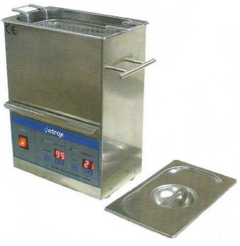
In the process of Ultrasonic Cleaning, the material that is desired to be cleaned, is put in the solution and the process is carried out by sending ultrasonic sound waves to the solution. High frequency sound waves are used to produce approximately 30.000 times higher and lower pressure changes.
